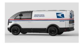
Also in February, the Postal Service detailed its plans to test the Canoo model Lifestyle Delivery Vehicle (LDV) 190. The Canoo LDV 190 is a battery electric commercial off-the-shelf vehicle with almost 172 cubic feet of cargo space. USPS states that the purpose of this test is to determine how the vehicle performs on carrier routes currently serviced by Long Life Vehicles (LLV), Flexible Fuel Vehicles (FFV) and Mercedes Metris vehicles.
